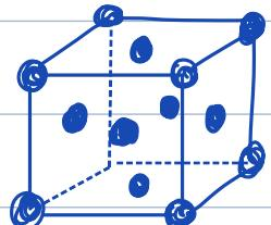
$$N = 8 \times \underbrace{\frac{1}{8}}_{\text{Sommets}} + 6 \times \underbrace{\frac{1}{2}}_{\text{faces}} = 4$$
