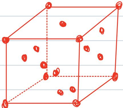
$$\begin{aligned} \text{On a } N &= \underbrace{8 \times \frac{1}{8}}_{\text{ sommets }} + \underbrace{6 \times \frac{1}{2}}_{\text{ faces }} + \underbrace{\frac{1}{4}}_{\text{ sites T}} \\ &= 8. \end{aligned}$$
